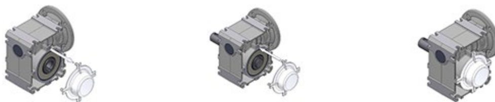
Figure 15: Disassembly and assembly of the cover cap
